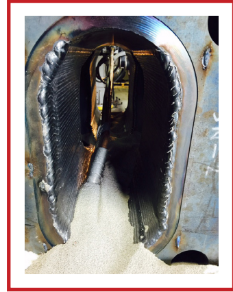
BOP CAVITY RAM WELDING
